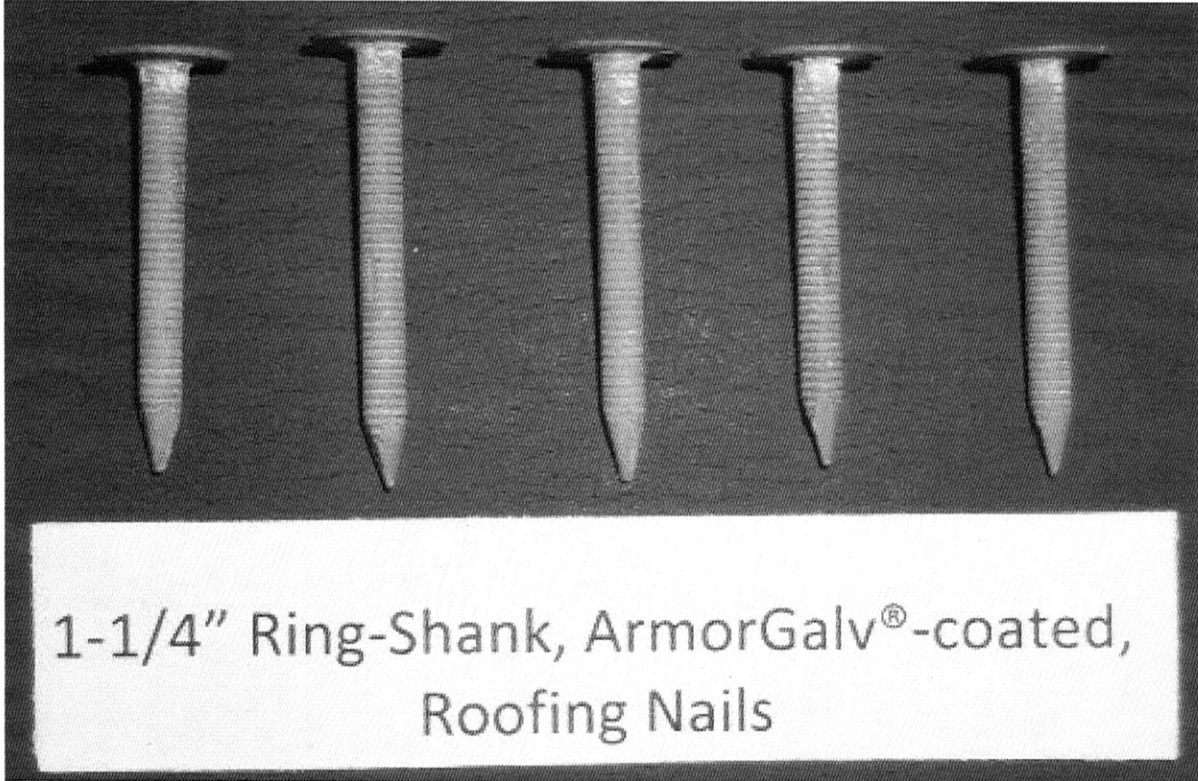
Photograph 5 1-1/4" Ring-Shank, ArmorGalv ® -Coated, Roofing Nails (After)
