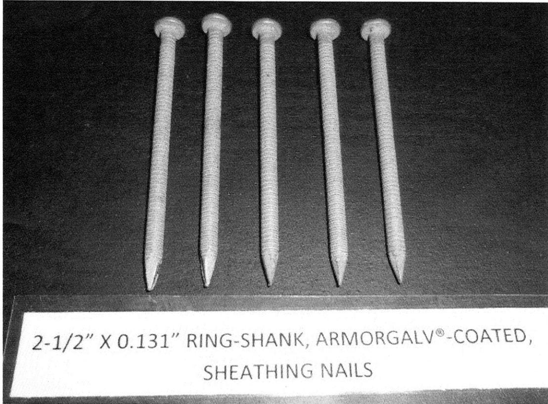
Photograph 2 2-1/2" x 0.131" Ring-Shank, Armorgalv ® -Coated, Sheathing Nails (Before)
