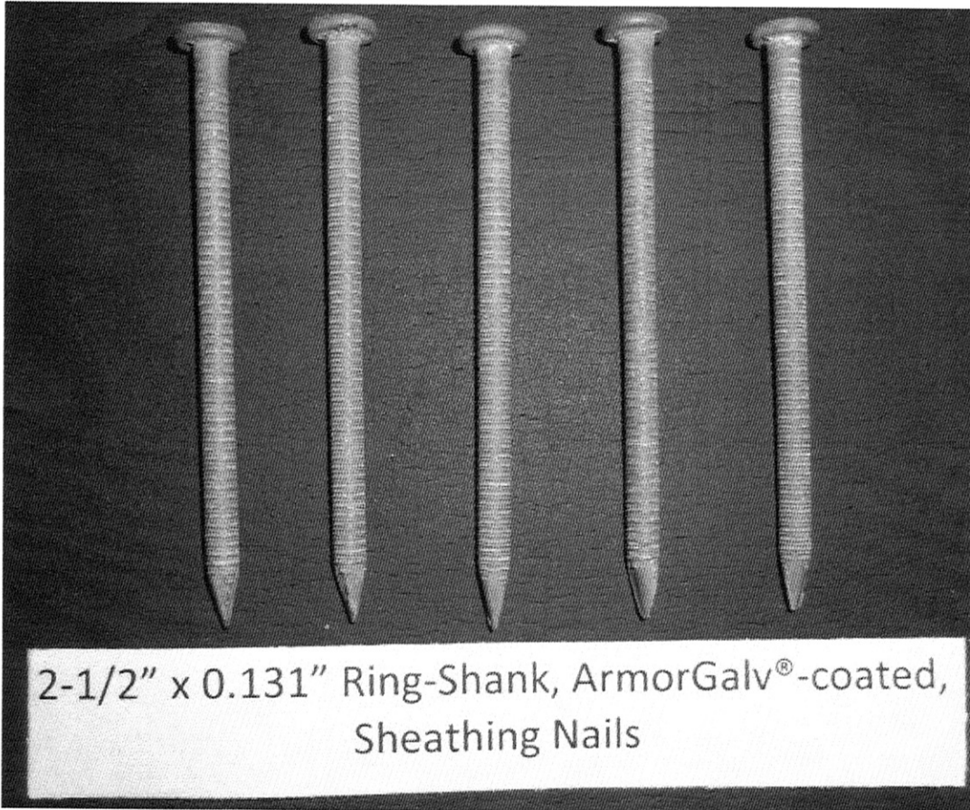
Photograph 6 2-1/2" x 0.131" Ring-Shank, ArmorGalv®-Coated, Sheathing Nails (After)
