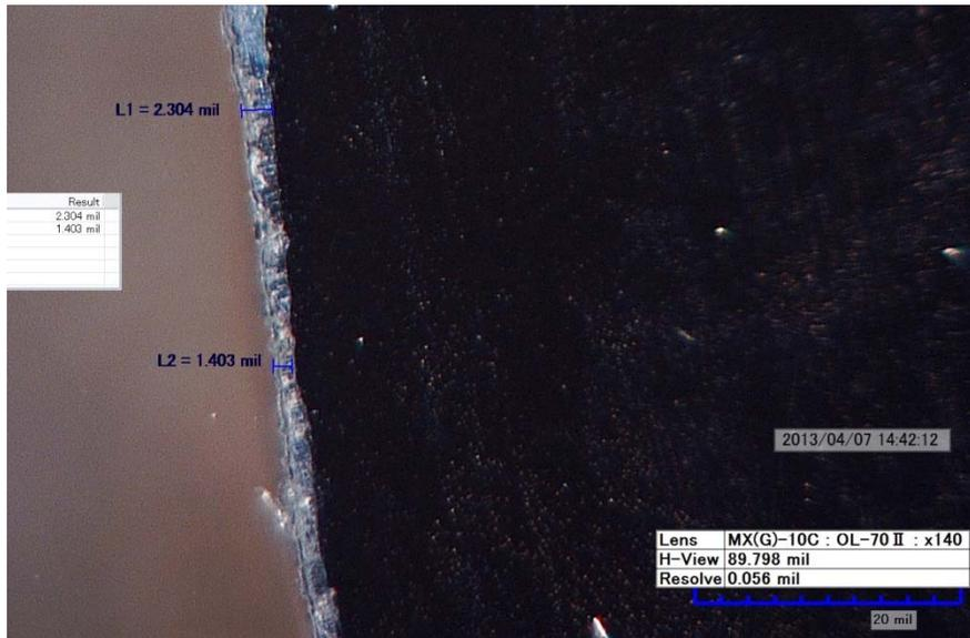
Figure 5 Unexposed specimen of ArmorGalv<sup>®</sup>
