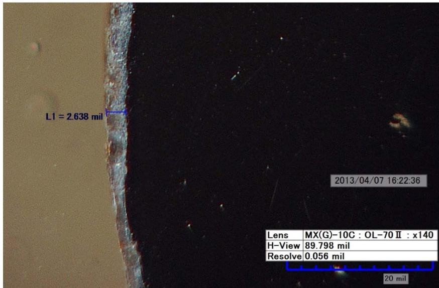
Figure 6 ArmorGalv<sup>®</sup> after 3000 hours in salt fog environment
